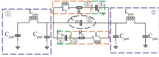
Fig. 3 Equivalent circuit of anti-parallel Schottky diode
