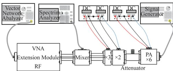
Fig. 7 Sub-harmonic mixer performance measurement platform for 0.825 THz
