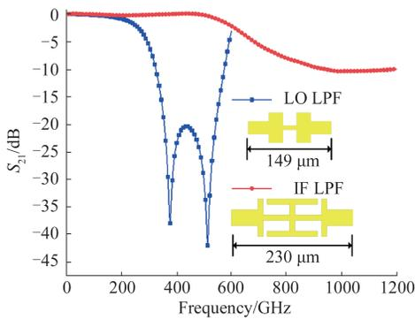
Fig. 6 Comparison of two different IF LPFs
