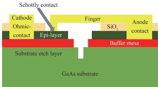
Fig. 1 Three-dimensional cross-sectional view of Schottky diode
