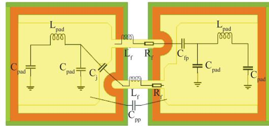
Fig. 2 Top view of anti-parallel Schottky diode
