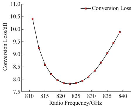
Fig. 5 Simulated 0.825 THz sub-harmonic mixer performance
