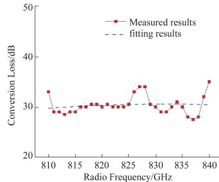
Fig. 8 Measured 0.825 THz sub-harmonic mixer performance
