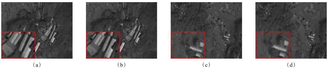
Fig. 11 (a) and (c) are the LWIR raw images; (b) and (d) are correspondingly noise-removed images
