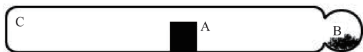
图 2 样品 Hg 压下封管高温退火示意图 注:A 是 HgCdTe 样品片,B 是退火源(Hg),C 是石英管 Fig. 2 Schematic diagram of thermal annealing under Hg pressure Note: A is HgCdTe sample, B is annealing source(Hg), C is Quartz tube
