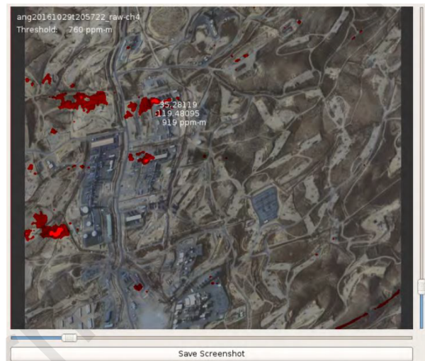
图4 AVIRIS-NG 机上实时甲烷测绘图 Fig. 4 On-board real-time methane mapping of AVIRIS-NG
